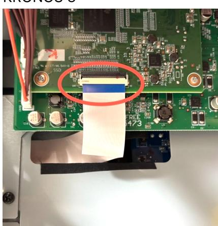
A photograph of the KRONOS 3 mainboard with the original FFC being removed. A red circle highlights the connector. | <p>Lift the black locking tab on the KRONOS mainboard connector.</p> <p>Carefully remove the original FFC.</p> |
