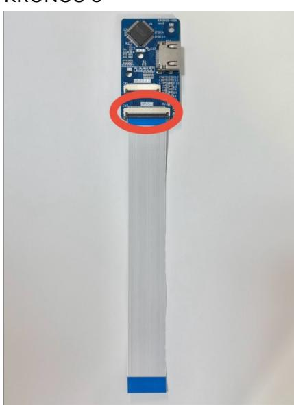
A photograph of the KRONOS 3 mainboard. A red circle highlights the 40-pin FFC connector labeled "INPUT(3)". | <p>Use the appropriate connector for your KRONOS model.</p> <p>Lift the black locking tab of the connector labeled "INPUT".</p> <p>Insert the included FFC with the blue reinforcement film facing up (visible).</p> <p>Push the cable straight in, then lower the black lock to secure it.</p> |
