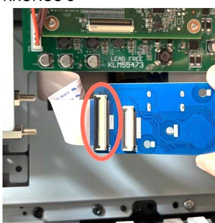
A photograph of the KRONOS 3 mainboard with the original FFC connected to the KRONOS-HDX board. A red circle highlights the connector. | <p>Use the appropriate connector for your KRONOS model.</p> <p>Lift the black locking tab of the connector labeled "THRU".</p> <p>Insert the original KRONOS cable with the blue reinforcement film facing up (visible).</p> <p>Lower the black lock to secure the connection.</p> |
